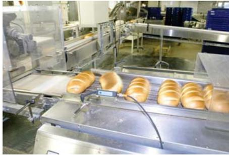
There are two common methods of oven chain lubrication. One method is to brush the oil on a moving chain as if painting the chain. The most efficient and consistent method of lubrication is with an automatic oiler. The volume and time of lubrication is pre-set. Make sure the automatic lubrication system has continual agitation to insure that the graphite stays in suspension for uniform lubrication.
